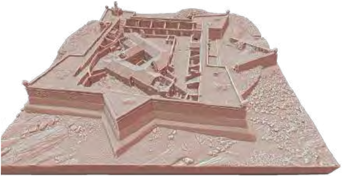
Fig.3 The closed watertight mesh model of Santa Maria de Insua monastery and the surrounding fortification prepared for 3D printing.
