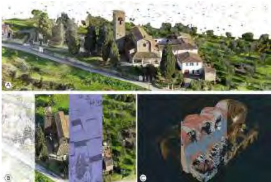
➔ Fig. 6 Capture phase through UAV (A) and photogrammetric processing using Metashape (B) and RealityCapture (C).
