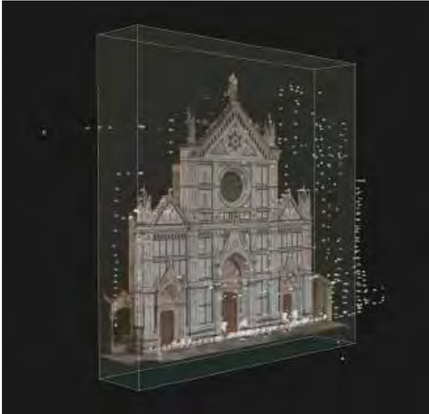
Fig. 2 Aerial photogrammetry by drone of the the façade of the Basilica di Santa Croce.
