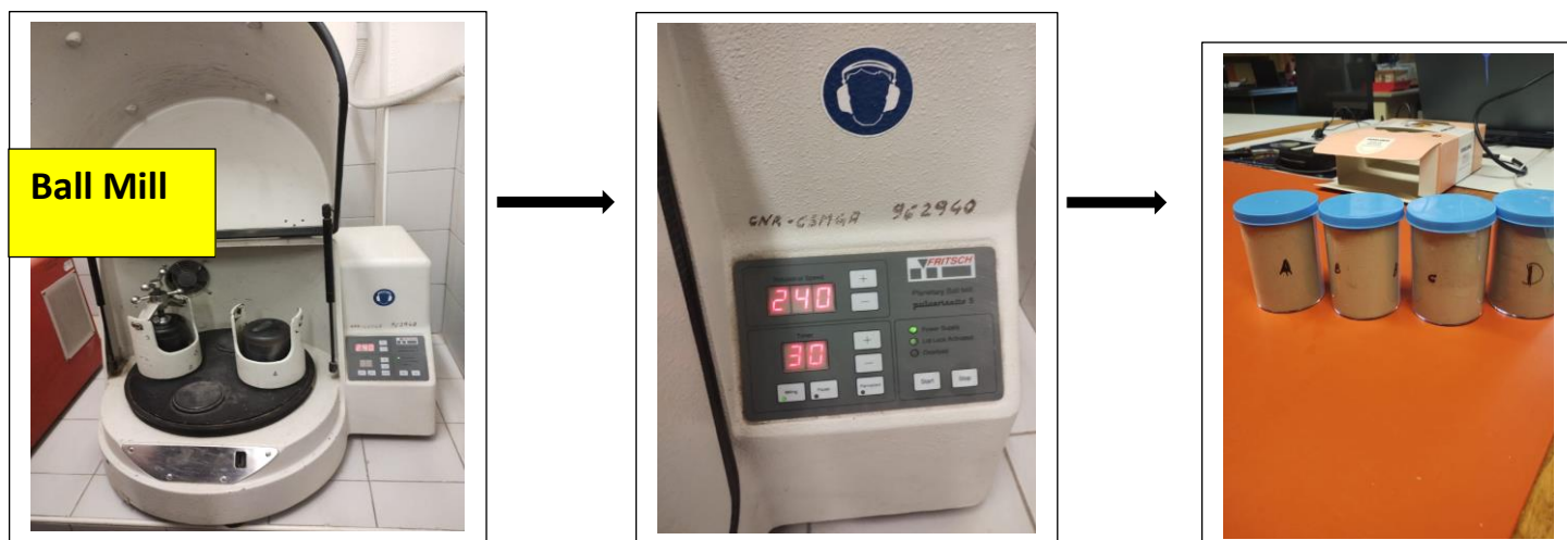
Figure III.6: Simplified Laboratory steps involved in rock sample preparations, from crushing to powder state
