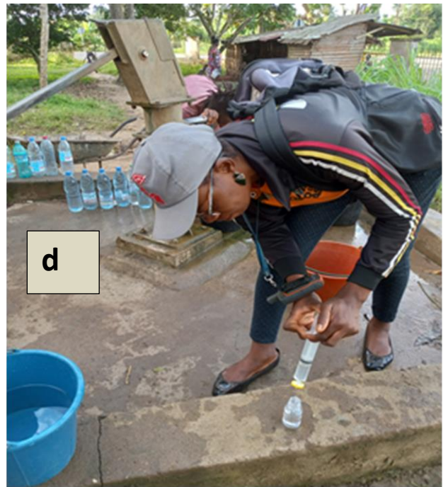
Noun River), (c) hand-dug wells, and (d) Sample filtration using the 0.45 \mu m cellulose filter
