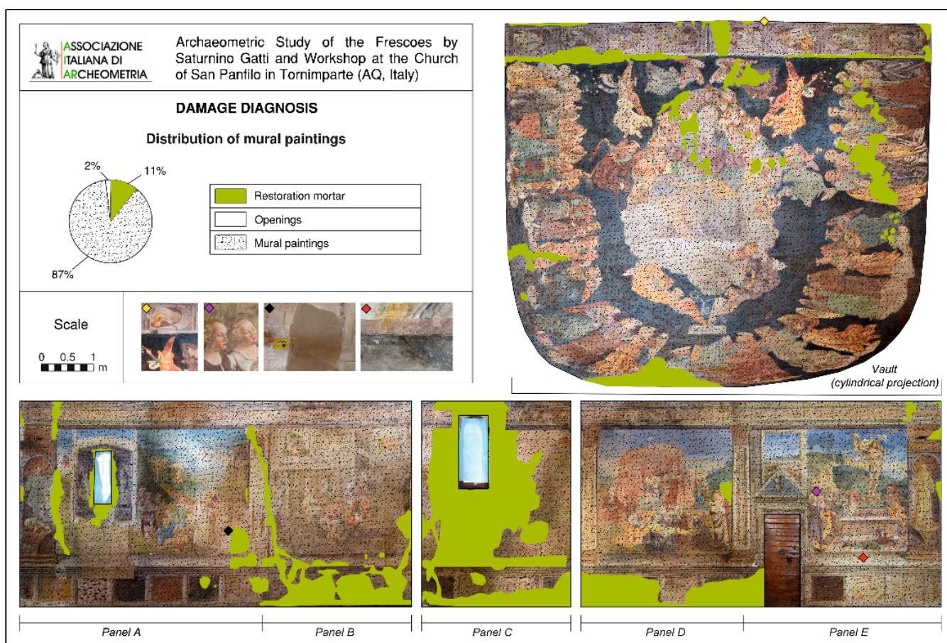
Figure 8. Distribution of geomaterials for the five panels and the vault of the apsidal conch of St. Panfilo Church in Tornimparte (AQ, Italy). Coloured dots indicate the position of the acquired pictures in the wall paintings.
