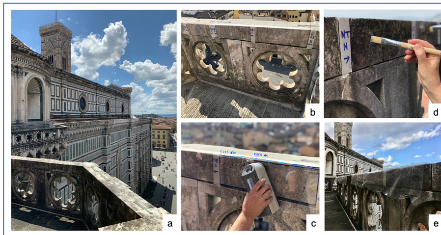
Fig. 1. The study sites for EOs treatment of marble of the Cathedral of Santa Maria del Fiore. (a) The external gallery running around the apses of the NW exposed façade; (b) a detail of the marble surface of the inner face of the openwork parapet of the SE exposed gallery; (c) colorimetric measurements on one selected SE area after application of the corresponding transparent sheet of acetate; (d) application of the reference solution (NT) by brush; (e) covering of the NW areas after treatment with transparent nylon sheets.
