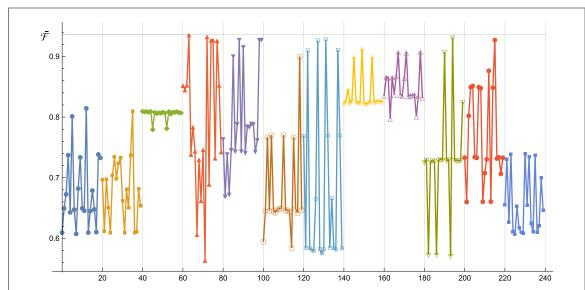
**Figure B10.** Training results for the Toffoli gate with a generator containing all one-qubit interactions and two-qubit interactions of the form  $J_{ij}(X_iX_j+Y_iY_j)$ . The initial conditions are chosen as in figure B8. The maximum fidelities obtained are  $\mathcal{F} \simeq 0.94$ , obtained in the c=3 sector.
