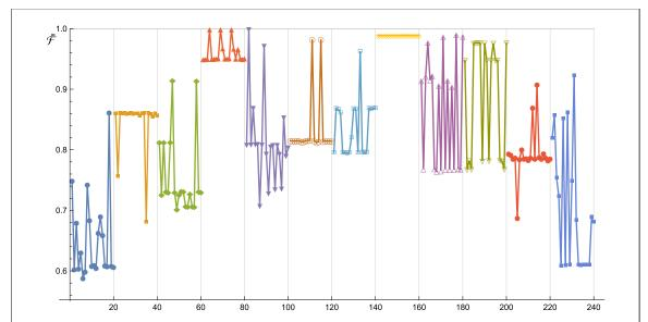
**Figure B9.** Training results for the Fredkin gate with a generator containing all one-qubit interactions and two-qubit interactions of the form  $J_{ij}^{(1)}X_iX_j + J_{ij}^{(2)}Y_iY_j$ . The initial conditions are chosen as in figure B8. The maximum fidelities obtained are  $\mathcal{F} \simeq 0.999$ , obtained in multiple instances c = 3 and c = 4 sectors.
