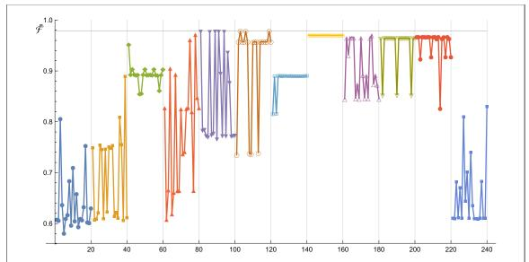
**Figure B11.** Training results for the Toffoli gate with a generator containing all one-qubit interactions and two-qubit interactions of the form  $J_{ij}^{(1)} X_i X_j + J_{ij}^{(2)} Y_i Y_j$ . The initial conditions are chosen as in figure B8. The maximum fidelities obtained are  $\mathcal{F} \simeq 0.98$ , obtained in the c = 4 and c = 5 sectors.
