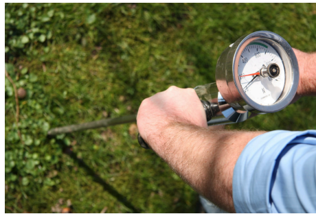
Figure 5: Soil penetration resistance was performed with an hand penetrometer EiJkelkamp
