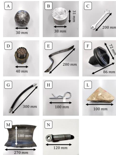
FIGURE 15. Images of the FODs used during the inspection in Linate selected from FAA document [2], [3].
