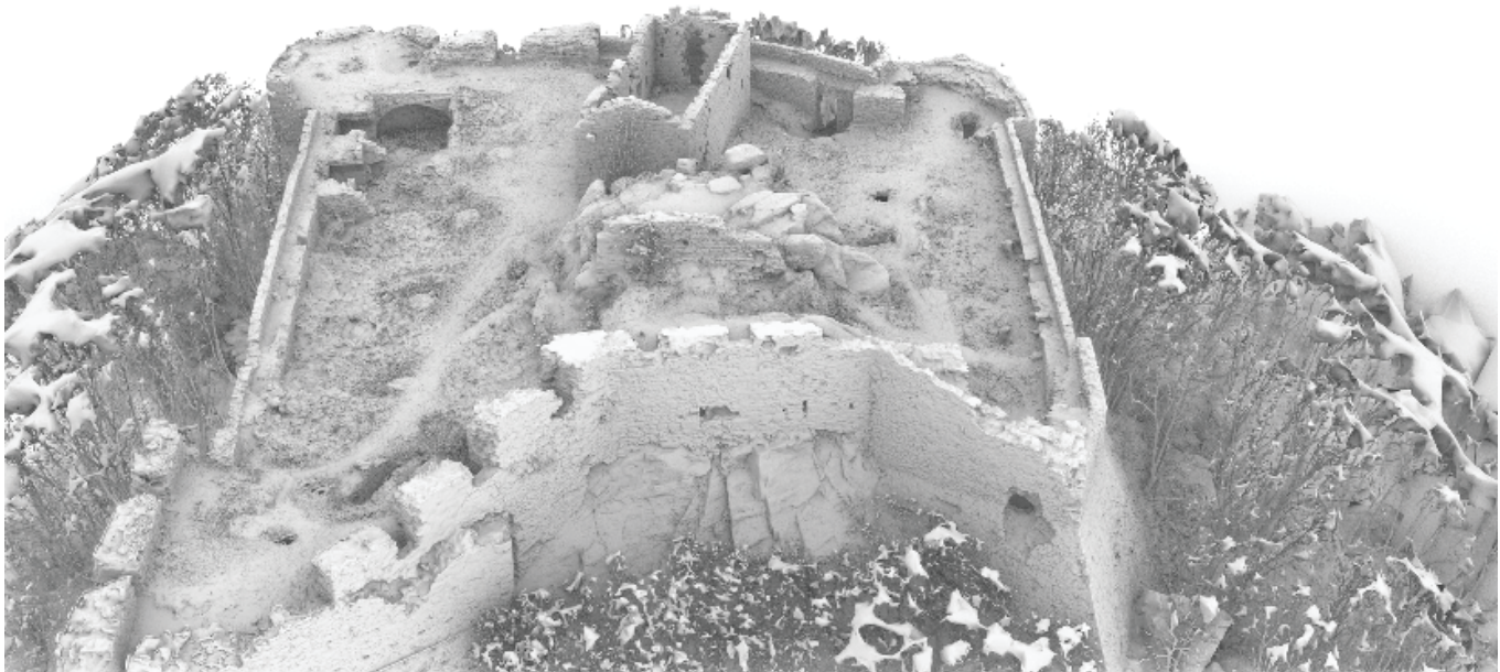
Figure 4. Three-dimensional model after the reconstruction integrated by laser scanner and photogrammetry.
