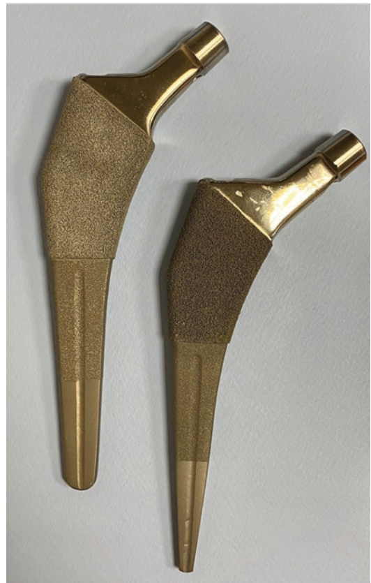
Fig. 9.5 Photograph of single-taper Anthology (left) and Anthology AFIT (right) femoral stems (Smith and Nephew, Memphis, TN, USA). The AFIT style stem allows for enhanced proximal fit with less chance for distal binding or so-called potting
