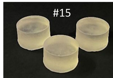
Figure 7 Elastic 50A specimens realized in triplicate. ID number according to Table 1 is reported.
