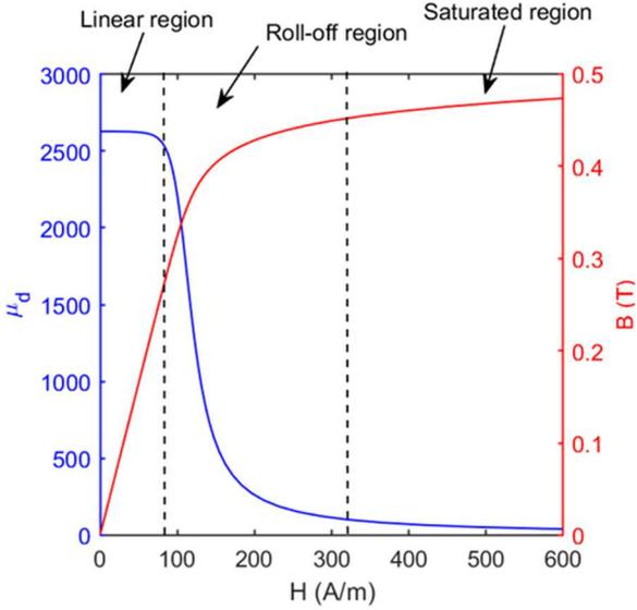
Fig. 3. Magnetization curve of a Mn-Zn ferrite. The red line represents the B-H curve and the blue line represents the related differential permeability profile. The three different operating regions of soft magnetic material are highlighted.
