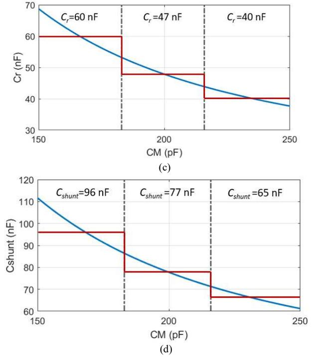
Fig. 2. Effect of coupling coefficient variations. (a) Resistive and reactive part of the impedance  $Z_R$ . (b) Resonant inductance  $L_r$  required for different coupling. (c) Required resonant capacitance  $C_r$ . (d) Required shunt capacitance  $C_{shunt}$ .
