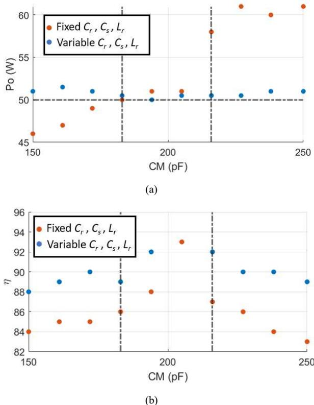
Fig. 5. Obtained simulation results. Red points represent the measurements of the system with fixed values. Blue points represent the measurements with the proposed control strategy. (a) Output power. (b) Conversion efficiency.
