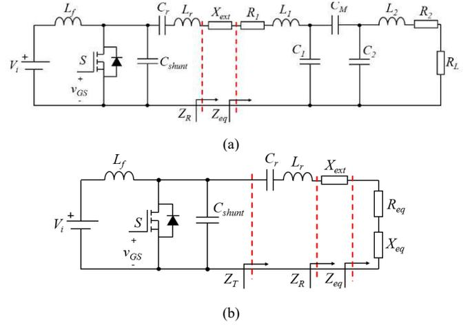
Fig. 1. Class-E inverter topology for CWPT. (a) Circuit with capacitive wireless power system. (b) Equivalent circuit.
