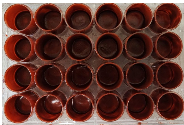
Figure 2. Acrylic 24-well plate brushed with prepared coatings.
