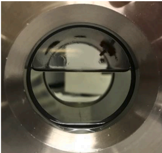
Fig. 4. Example of Propylene miscible in PAG oil.
