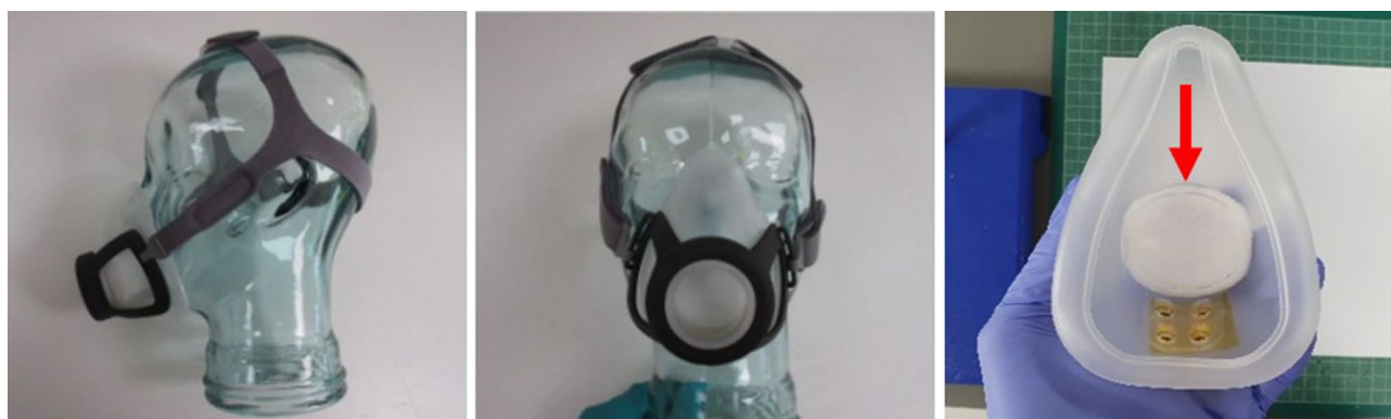
Figure 5. A filter held by a CPAP-type face mask was used to capture exhaled virus particles. The face mask, holder and head strap shown on a glass head in profile (left) and face on (center). An inside view of the face mask (right) with electrostatic filter (red arrow); holes at the bottom were sealed with tape.
