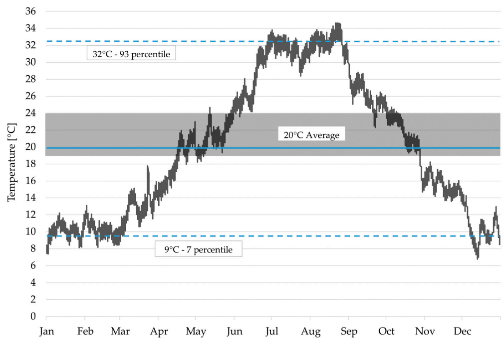
Figure 22. Trend of historic climate hourly values of T and statistical limits of 93rd and seventh percentiles in room X vs. the range recommended by the Italian D.M. 10.05.2001 [16] (gray band).
