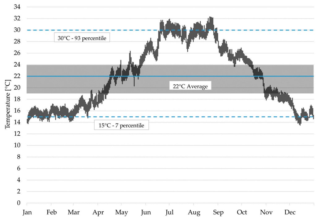
Figure 23. Trend of historic climate hourly values of T and statistical limits of 93rd and seventh percentiles in room XXII vs. the range recommended by the Italian D.M. 10.05.2001 [16] (gray band).
