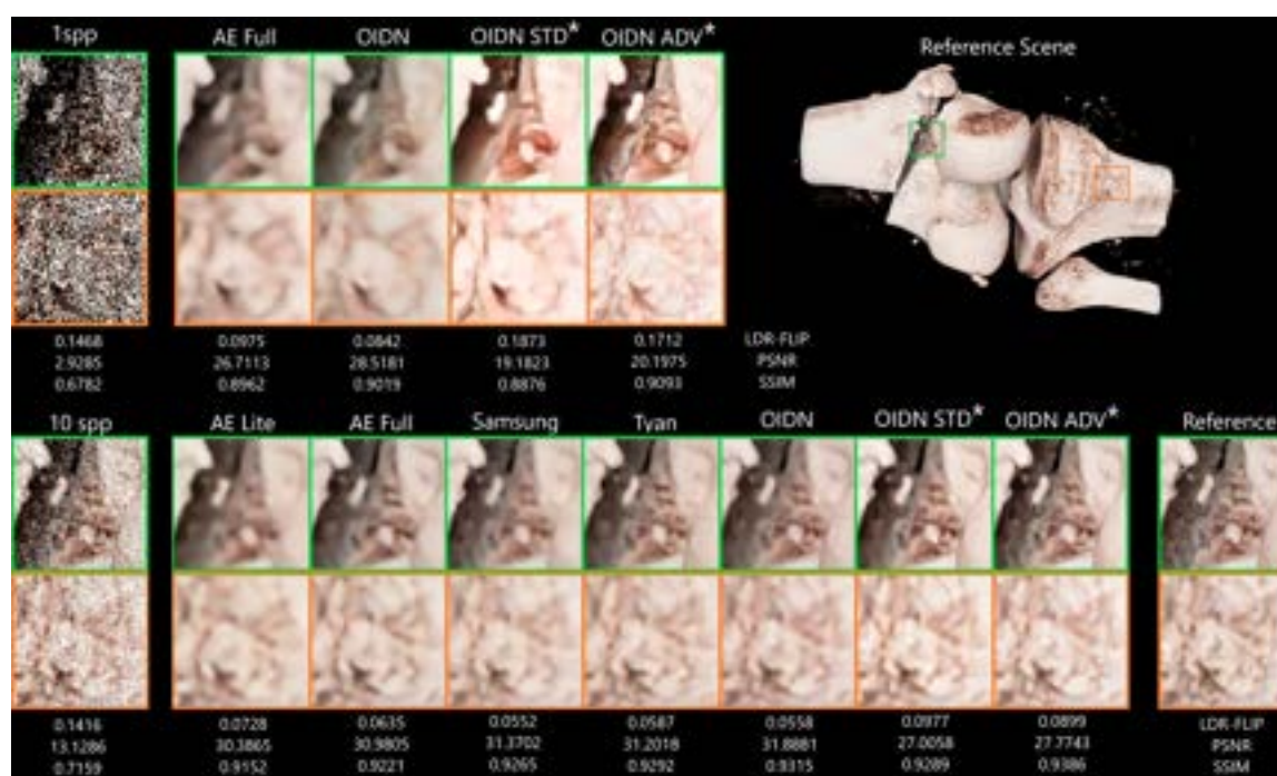
Figure 6. Visual comparison of denoising single-sample-per-pixel (1 SPP) and 10 SPP inputs for a scene predominantly composed of surfaces. The reference scene was generated from a CBCT scan of a broken knee (post-mortem) with 659 SPP. The upper row shows two crops, multiplied by 4, of denoising results using 4 different models with 1 SPP input, while the lower row displays results from 7 models with 10 SPP input. '*' indicates pre-trained models. Colored squares mark the cropped regions. The metrics reported under each model were calculated on entire image.
