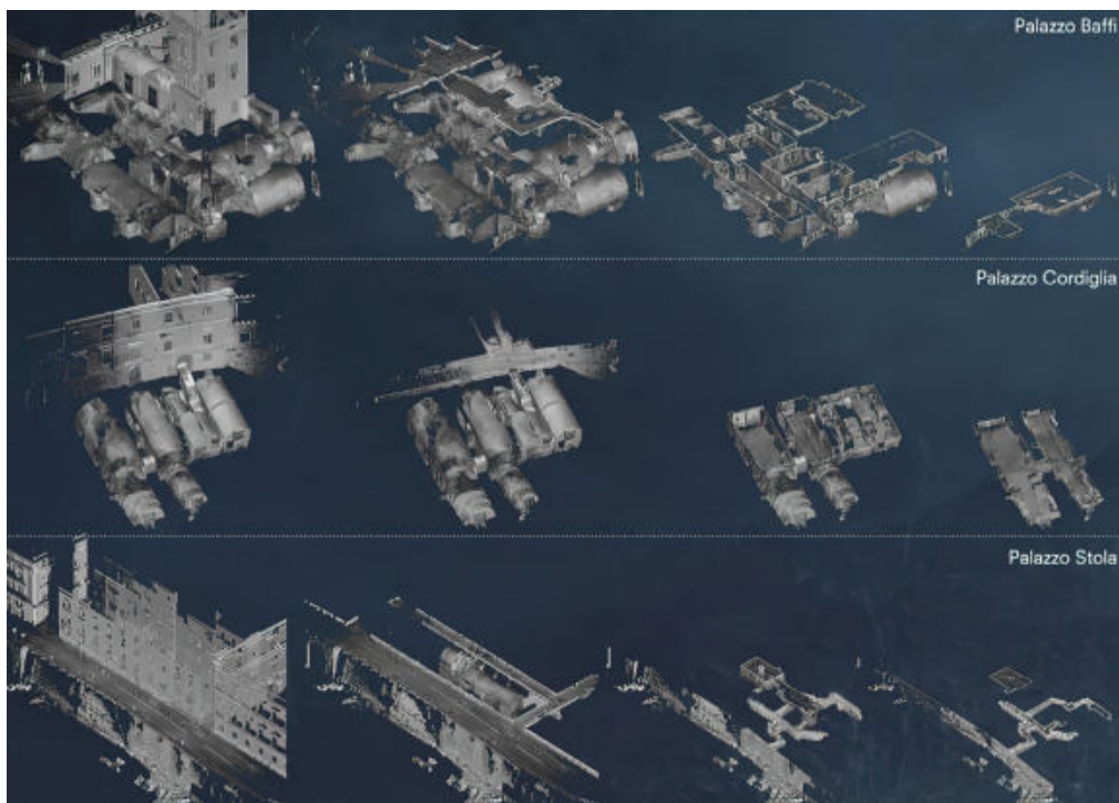
Fig. 5- Axonometry views obtained by cutting the point cloud model from Autodesk Recap at variable heights (Giada Germanà, 2022)
