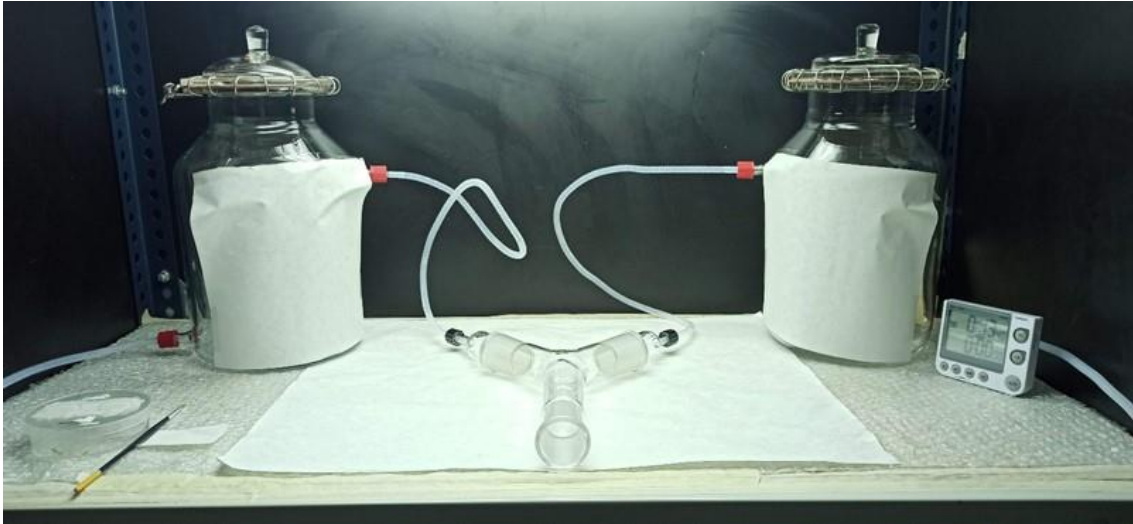
Figure 1. The Y-tube olfactometer used for behavioural assays. The jars were screened with a white sheet of filter paper to avoid the influence of visual stimuli.
