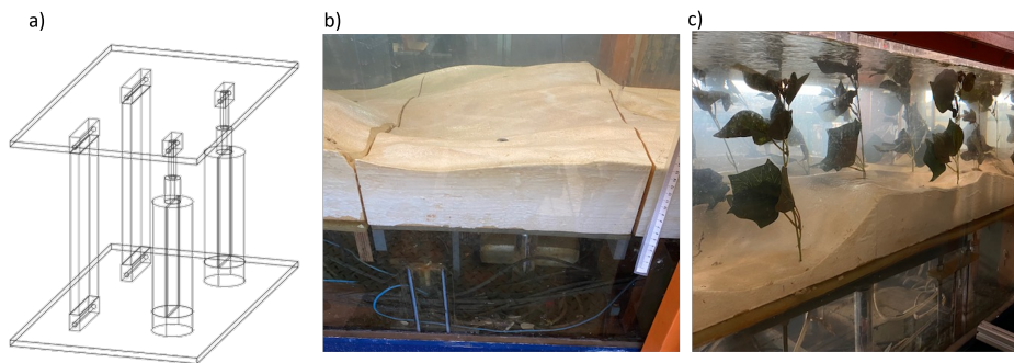
Figure 5.4: Instruments setup for measuring dune form drag and vegetation drag. a): a 3D sketch showing the shear plate with the two drag force sensors (DFSs) and two supports designed to restrict movements primarily in the horizontal direction; b) the shear plate connected to the fixed dunes model through the head plate; c) plants installed over the dunes and connected to the DFSs, which are positioned underneath the flume bottom.
