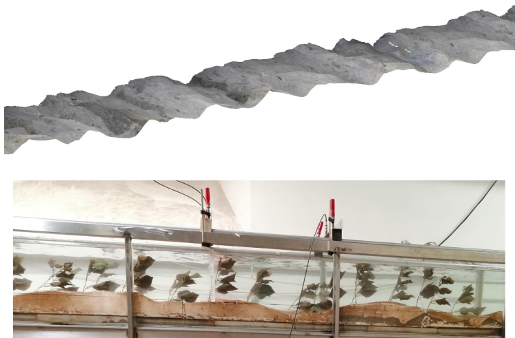
Figure 4.2: On the top, the DEM relative to the 12●4 setup. On the bottom, the corresponding fixed dunes model installed in the flume of the University of Florence.
