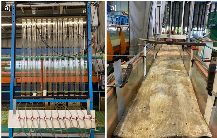
Figure 5.3: a) Eight piezometers were employed to measure the water surface elevation along the flume. A traverse system was installed above the piezometers, facilitating the movement of the ultrasonic sensor over them; b) the flume setup for HF experiments.
