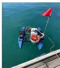
Fig. 1. Automated Surface Vehicle equipped with multispectral cameras and chemico-physical sensors.
