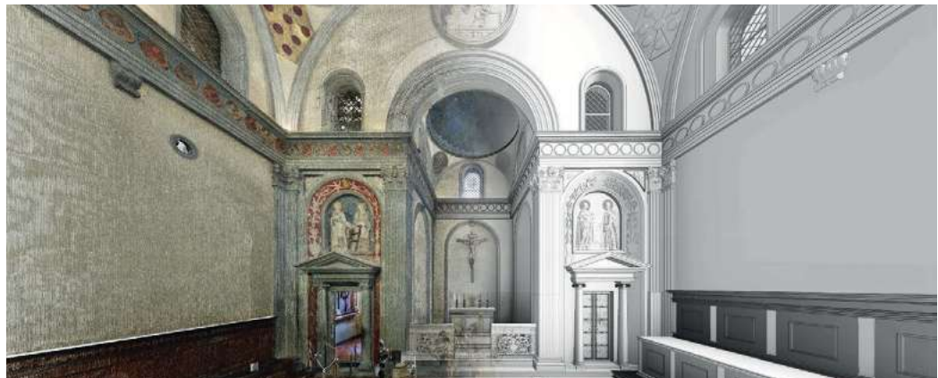
From the point cloud to the HBIM model of the Old Sacristy of San Lorenzo in Florence.
