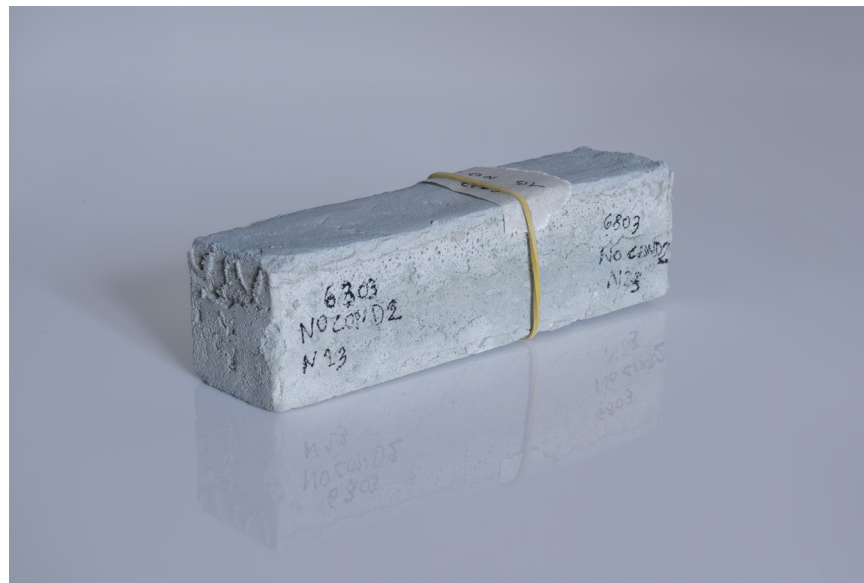
Fig. 3 - INERTIAL project: A sample of biomaterialized material produced for mechanical bending and compression tests. Standard dimensions: 160x40x40 mm (Photo credits: Cristian Betti).
