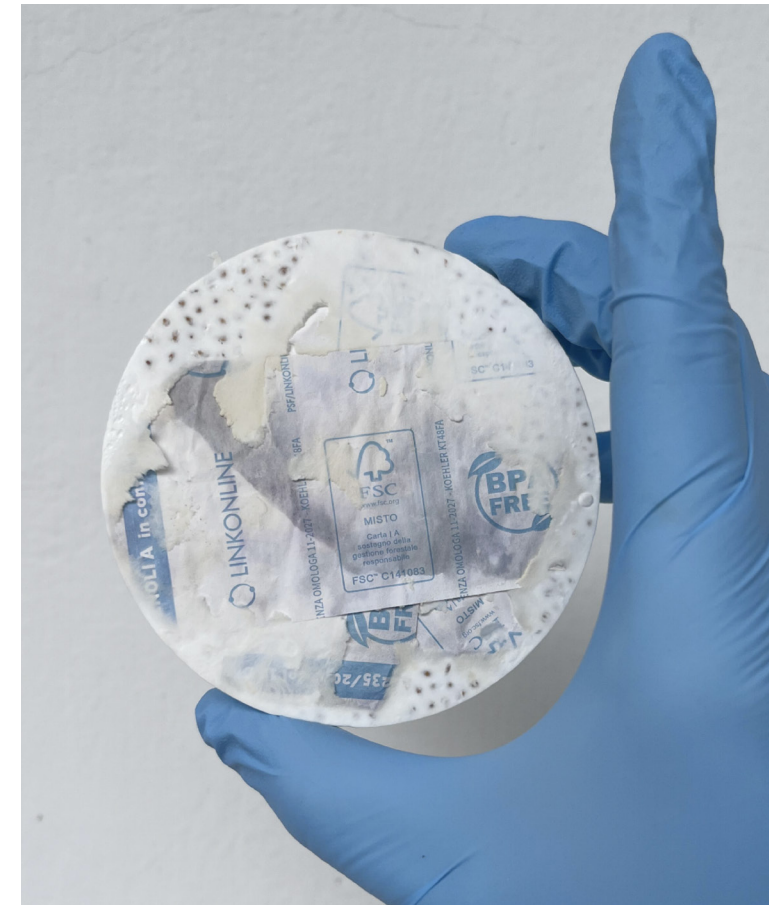
Fig. 2 - A sample of micocomposite material on a receipt substrate developed by students as part of the Material Beyond Materials III workshop (Credits: Rachele Moriconi).
