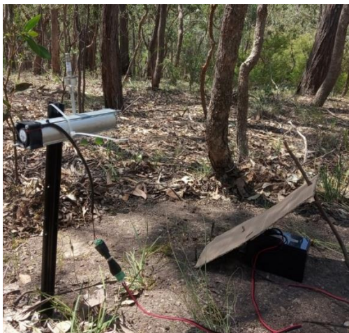
Figure 7. Picture of DBSS device with SPME fibre during the BVOCs sampling in Bunjil reserve, Phantom Hill (Victoria, Australia).
