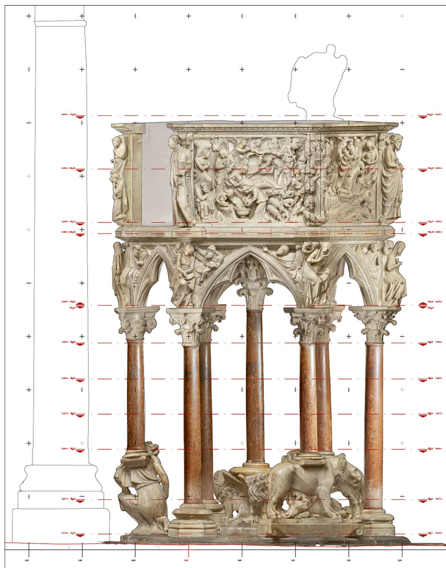
Fig. 7.2 Extract from the elevation drawing with orthoimage (GSD 0.005 m). Original scale 1:5
