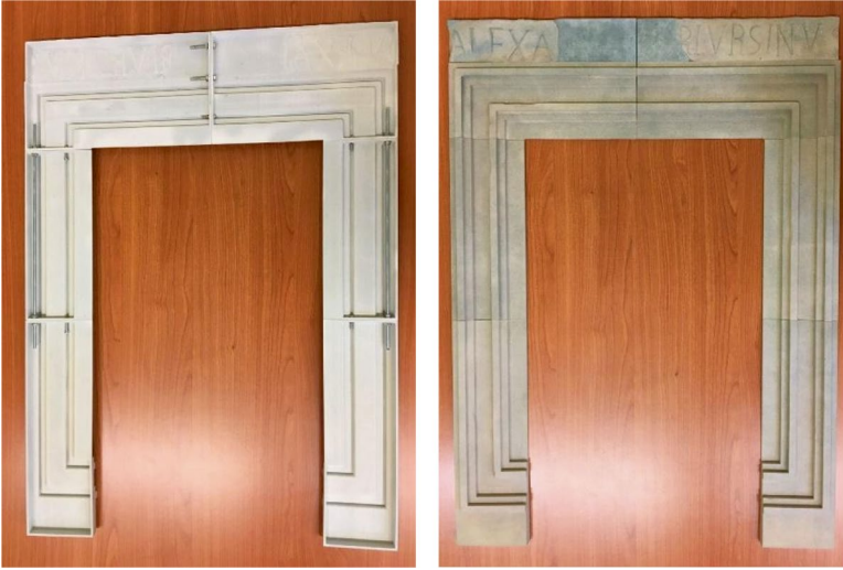
Fig. 26.4 3D-printed cornice (3:1 scale) of Palazzo Orsini in Amatrice
