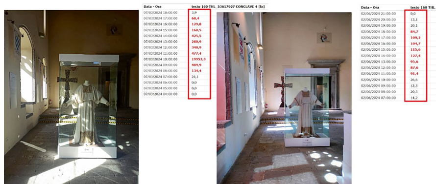
Fig. 10.7 Comparison between the values of illuminance before and after the mitigating emergency intervention in two sunny days
