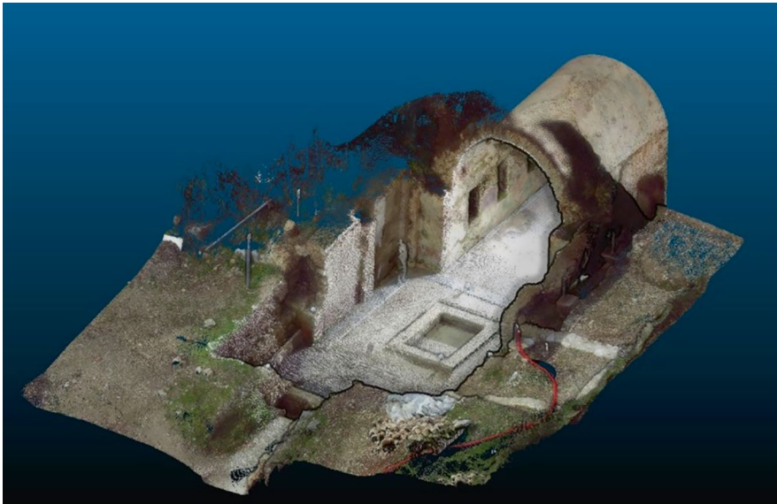
Fig. 9.1 3D point cloud processing with textures
