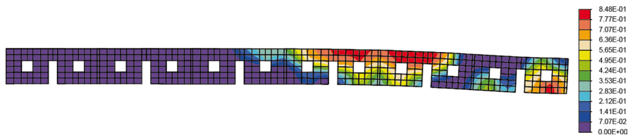
Fig. 12.7 Distribution of the damage variable D at the end of the analysis
