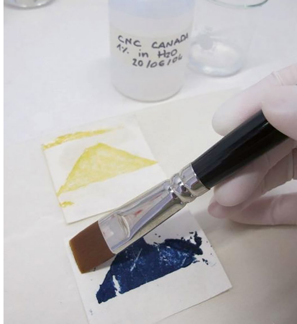
Fig. 24.5 Application of CNC on test samples of Japanese paper realised by ukiyo-e print technique
