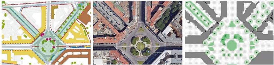
Fig. 4.3 Detailed map of analysis, aerial photo of the current status and ENVI-met modelling of the application of NBSs (i.e., raingardens, street trees and permeable paving systems) on one of the sample areas. (Elaboration by Federica Lecci)
