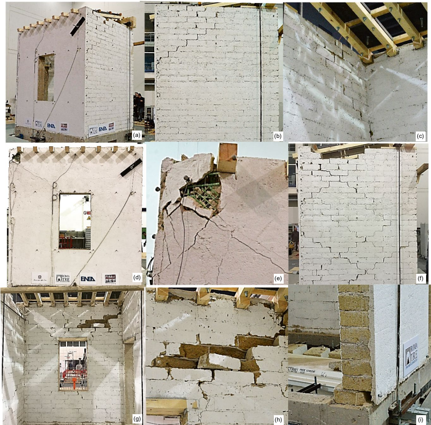
Fig. 18.7 Damage of the reinforced prototype after NCR22 ( a_{\max} = 1.78 g)
