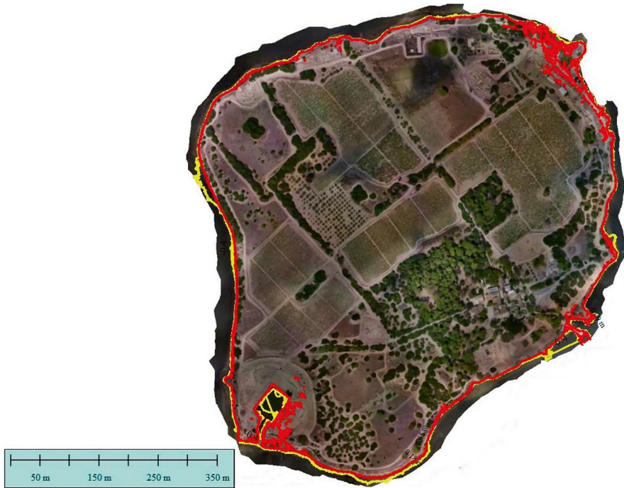
Fig. 16.6 2100 A.D. coastline projection for the RCP 8.5 + VLM scenario for Motya island: in yellow (continuous line) the current coastline, in red the coastline projection (continuous line) with its minus/plus uncertainty (dashed lines)
