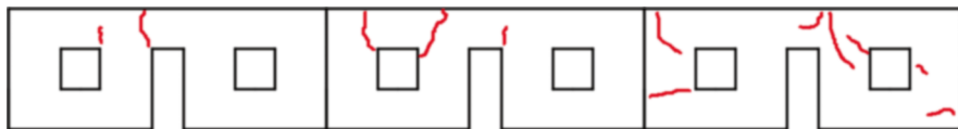
Fig. 12.8 Schematic representation of the real damage occurred at the last three dwellings. [Adapted from Camós et al., 2014]
