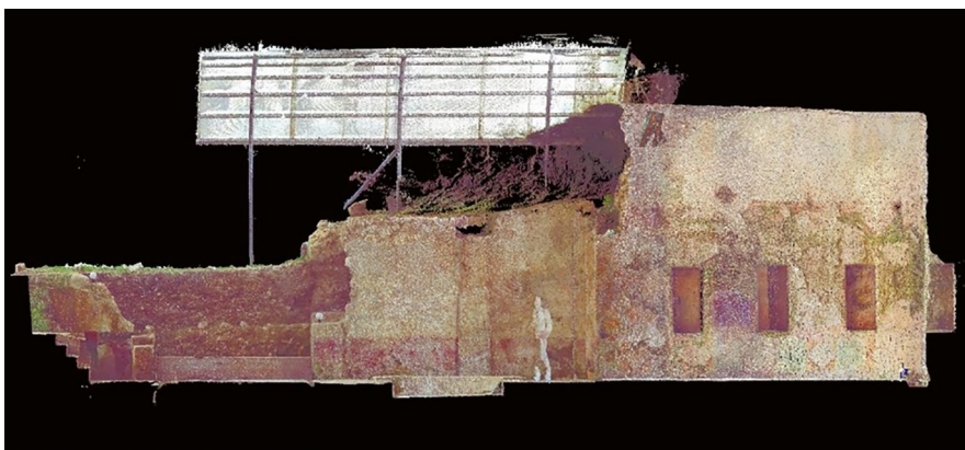
Fig. 9.8 3D processing from point cloud—longitudinal section
