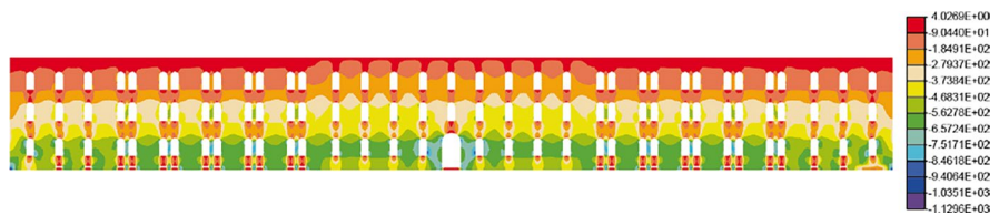
Fig. 12.12 Distribution of the vertical stress, \sigma_y [kN/m 2 ], for load combination 1
