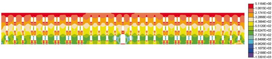
Fig. 12.15 Distribution of the vertical stress, \sigma_y [kN/m 2 ], for load combination 2
