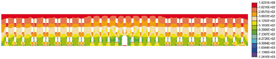
Fig. 12.14 Distribution of the minimum principal stress, \sigma_{min} [kN/m 2 ], for load combination 1
