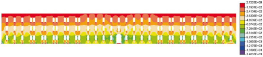
Fig. 12.17 Distribution of the minimum principal stress, \sigma_{min} [kN/m 2 ], for load combination 2
