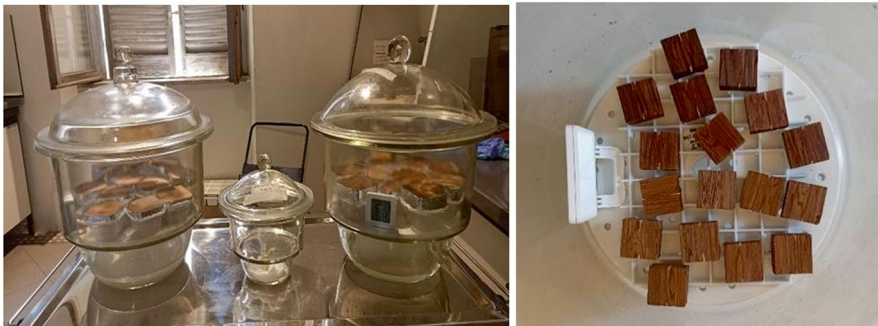
Fig. 24.8 Test samples realised with Dunarobba ancient wood
