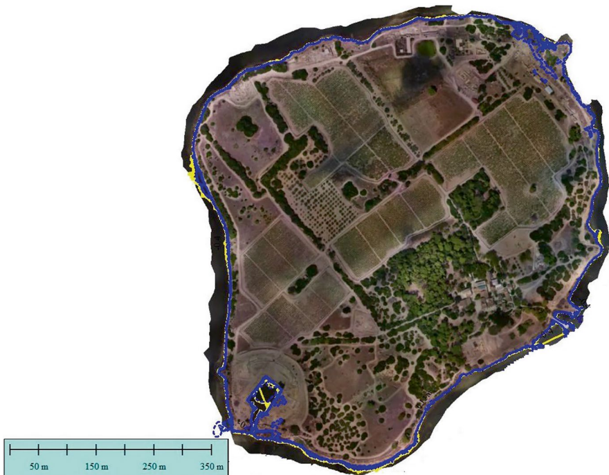
Fig. 16.5 2100 A.D. coastline projection for the RCP 2.6 + VLM scenario for Motya island: in yellow (continuous line) the current coastline, in blue the coastline projection (continuous line) with its minus/plus uncertainty (dashed lines)
