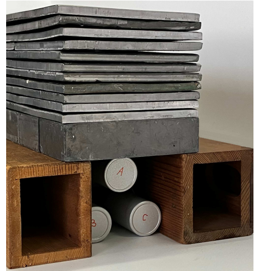
Figure 7. (Color online) A photo of the GM arrangement used to reproduce Rossi's curve. The tubes are kept on the vertices of an equilateral triangle with a side length of 40 mm thanks to properly machined plastic spacers inserted between them. Lead sheets (for a total thickness of 91 mm in this case) were placed horizontally above the tubes, as shown, resting them on lateral supports made of wood.
