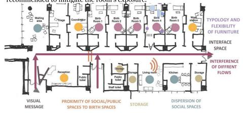
Figure 1. Preliminary project layout and critical aspects. The colour of the big dots is related to the writing of the same colour (© TESIS -DIDA)
