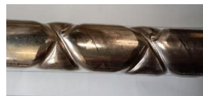
Figure 2. Details of the corrugation of pipes (a) T1 (b) T2
