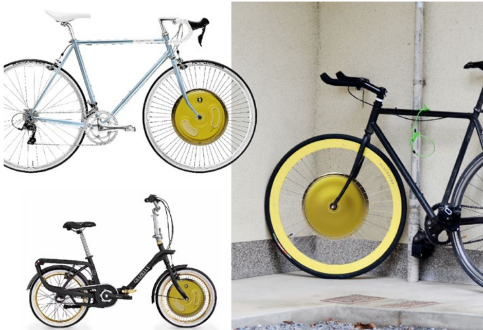
Figure 1. The conversion kit is compatible with bicycles ranging from 20 to 29 inches in size. Design by Michele Marco Tizza - IDEE Lab.
