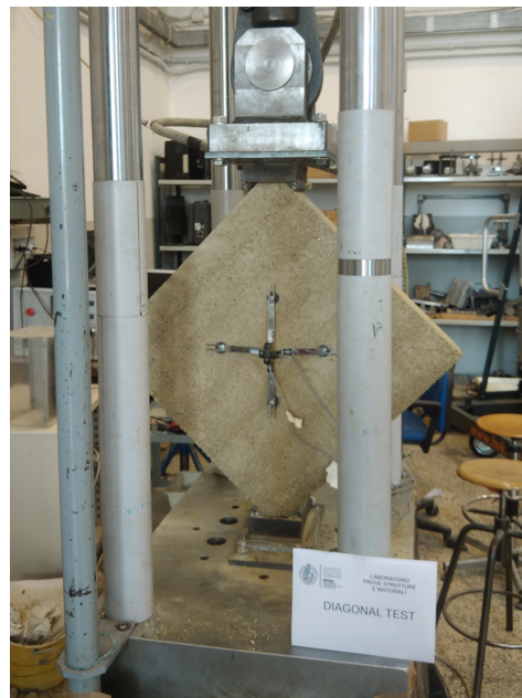
Figure 12. Setup for the diagonal compression tests.
