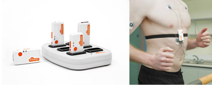
Figure 2.7: Shimmer3 devices used for EDA and ECG acquisition.
