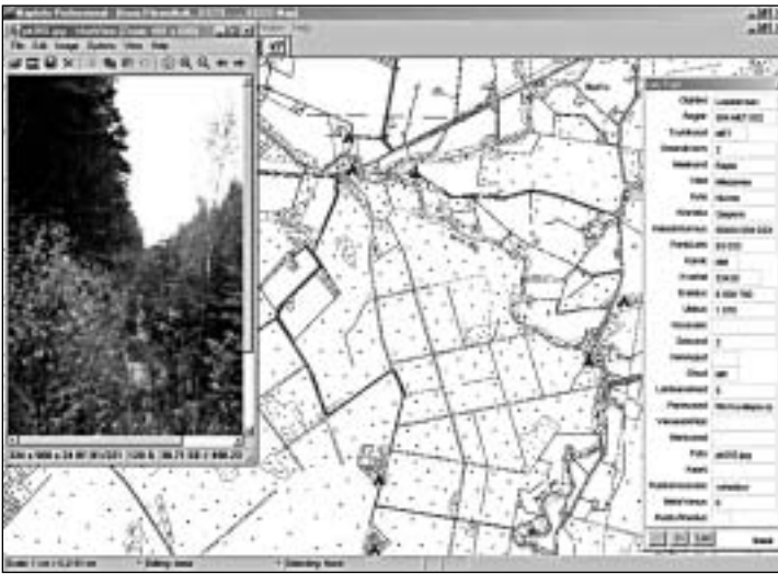
Figure 2. Map window in the MapInfo GIS software showing the photo of the object and the data table record
