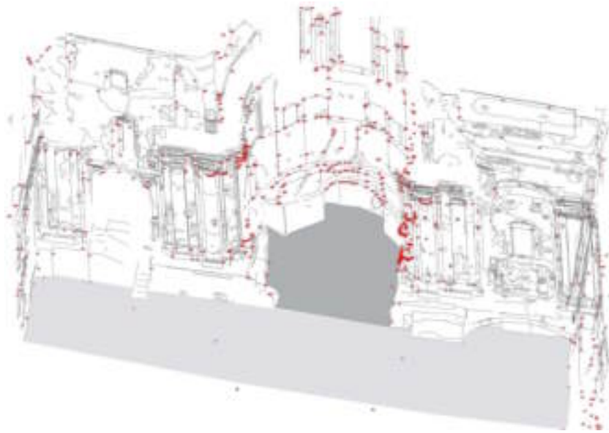
Figure 1. Matching of topographic data (red points) and photogrammetric restitutions
