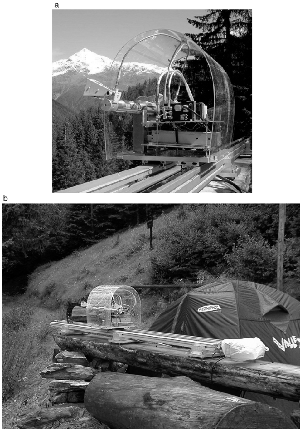
Figure 6. The portable version of LISA used in the test site: (a) detail of the antennas and (b) field arrangement of the instrumentation.
