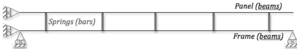
Fig. 2. Simple FE model of wooden panel with frame linked with springs
