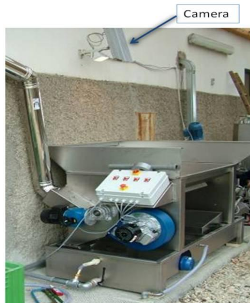
Figure 2. Positioning of the CMOS uEye camera.
