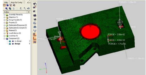
Figure 10: Mesh generation and loads and constraints assignment
