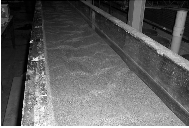
Fig. 3. Bed forms at equilibrium configuration without seepage
