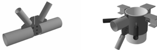
Figure 5. Views of a typical joint of roof and floor trusses, and a truss-column-longitudinal beams connection.
