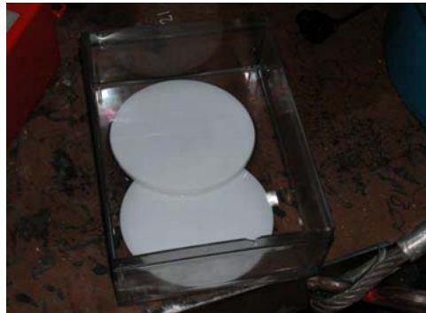
Figure 3. Two Teflon disks during the lubrication phase
