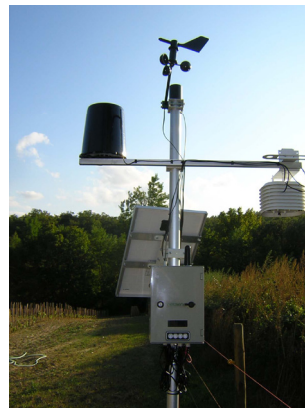
(b) VineSense GPRS Gateway with Weather Sensors
