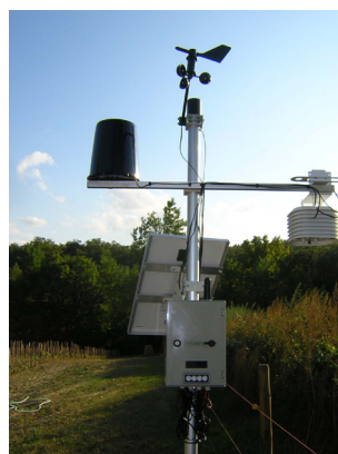
(b) VineSense GPRS Gateway with Weather Sensors
