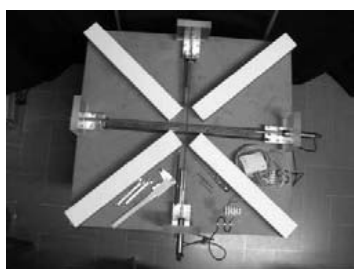
Fig. 17 – The “deformometric kit”, purposely designed and built for monitoring this kind of shields. Four Plexiglas feelers slide freely on perpendicular low friction rails.
