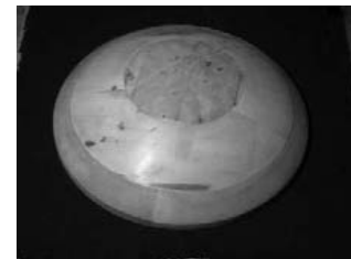
Fig. 6 – The wooden mould shaped (by turning) as a spherical section, to be used for assembling the lamellae.
