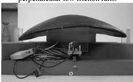
Fig. 19 – The shield 408 mounted on the apparatus: side view, showing the shorter (“horizontal”) diameter. The 4-channel data-logger has self sufficient batteries, which also supply power to the transducers at moment of measurement, which in this case was set every 15 minutes.
