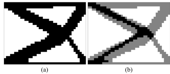
Figure 7 (a): Topology obtained by hybridization of mono-objective topology shown in Fig 3. (b): Operational zone of the geometrical contradiction.
