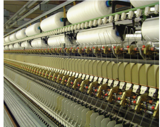
FIGURE 2: (a) Example of output obtained by means of the OFDA instrument: statistical distribution of the fineness. The mean value is assumed as the fineness parameter. (b) Ring frame machine used in the work.
