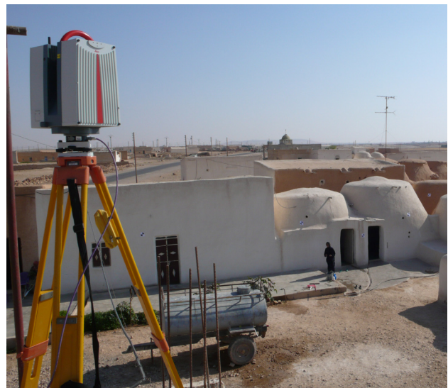
Figure 1. Joub Maadi: view during the 3D scanning survey
