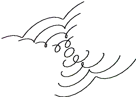
FIGURE 5. A circular orbit under the influence of a uniform current \kappa . To the left and backmost: a favourable current ( \kappa > 0 ). To the right and foremost: a current working against the wave ( \kappa < 0 ). Notice that the case of irrotational Stokes waves corresponds to the loop just behind the closed circle, in which case the drift is rightward. As \kappa decreases the drift becomes negative and leftward on this side of the closed orbit.
