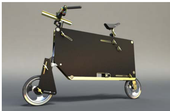
Fig. 1. Measuring model. This prototype has been used to test different postures.
