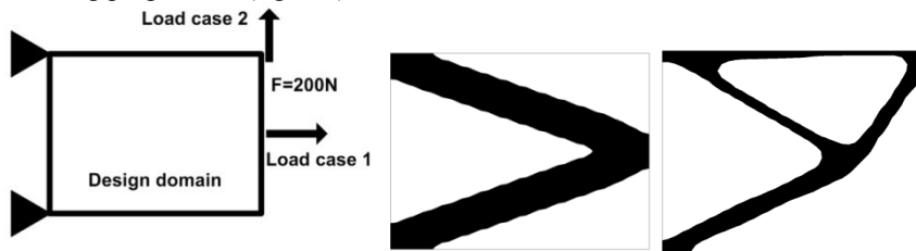
Fig. 2.5 The plate is fully constrained at the corners on the left edge and the forces are alternatively applied on the middle and the upper point of the right edge (left). Topologies obtained through mono-objective optimization under load case 1 and density threshold = 0.27 (middle) and under load case 2 and density threshold = 0.83 (right).
