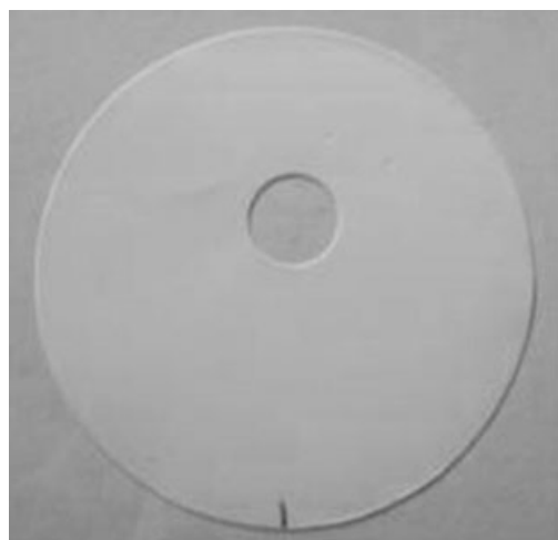
Figure 2. Mixed cellulose ester sample holder for standard and sample positioning in the ED-XRF system with the SDI configuration.
