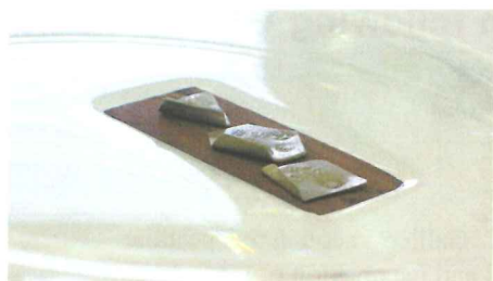
Fig. 2. A thin plate of ebony, also bearing some small weights, can float in water, but it sinks when touched.
