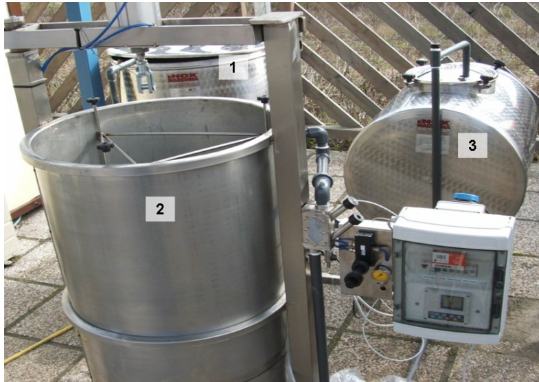
Fig. 1. 500 litres pilot plant for OMW semi-continuous process: OMW collecting tank (1); biofiltrating main structure (2); treated OMW collecting tank.
